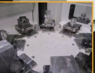
2015 - Introduced 10-station APC (field expandable) pallet pool in tandem with our Mycenter-HX250iG. Ultra-compact footprint, it's designed for high-production and multi-varied component machining.
